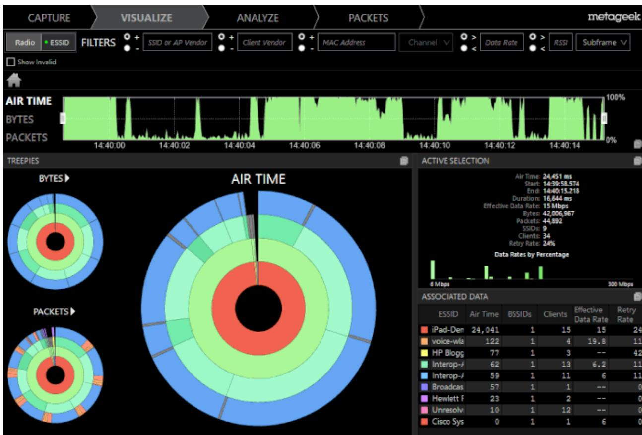
The darker yellow in the background represents all frames in the capture, while the brighter yellow in the foreground of the graph represents the data currently in view after navigation and filters have been applied. Sometimes a capture may have a dark yellow without any filters applied. This means some of the frames were corrupted and are invalid for reliable display. To see them in the graphs add a check to the **Show Invalid** checkbox in the filter bar.
