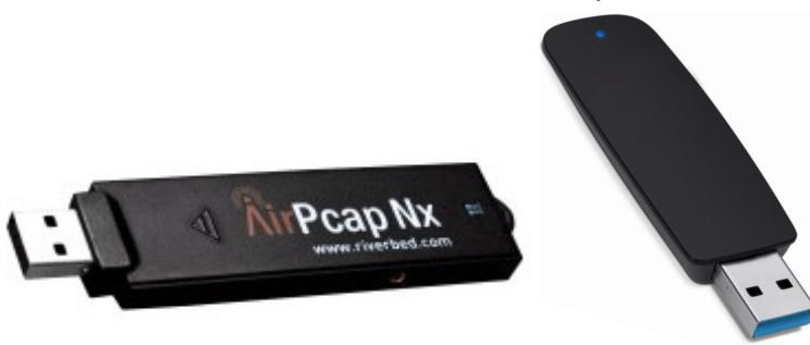
To begin, connect your device to your computer's USB port and open Eye P.A. Click the **Start** tab at the top of the screen. Here you will select the device that you would like to capture with, as well as the band and channel.
